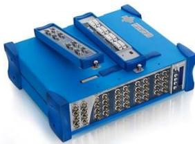
The Xpod modules add signal conditioning to the OR36 and OR38 in a smart and field operation driven design. These 8 channel conditioners can be added, removed and exchanged between the analyzers in a few seconds. Moreover, the lateral side clipping, leaves the BNC input connectors free to be used as classical ICP<sup>®</sup>/AC/DC/Float inputs.
