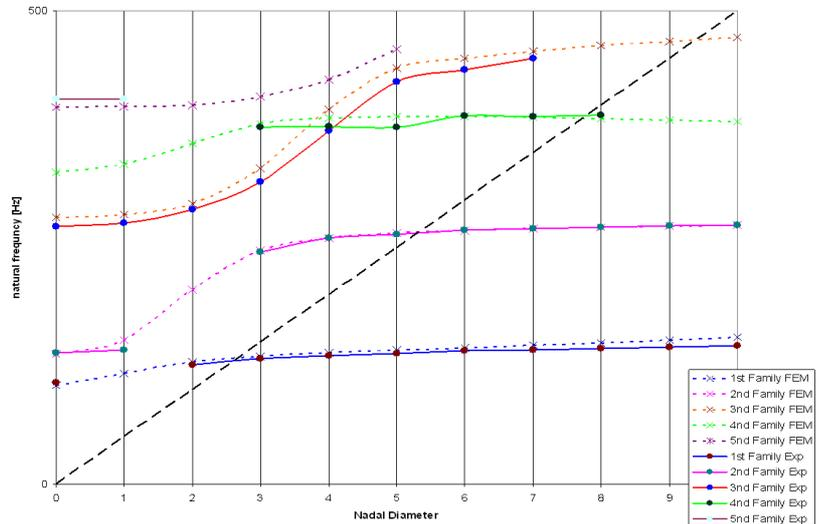
Interference diagram FEM-EXPERIMENTAL
