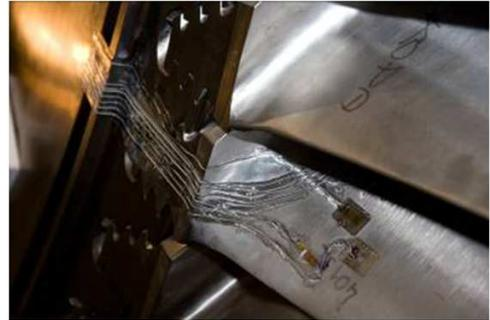
Strain gauges on a blade
