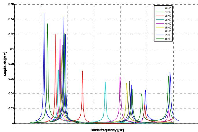
*Forced response analysis with blade resonance frequency on the X-axis.*
