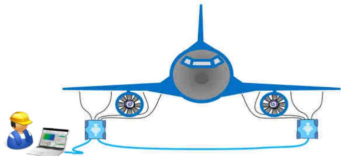
different possible configuration. For example, this flexibility allows to highly reduce the cable length by distributing the instruments along the structure under test.
