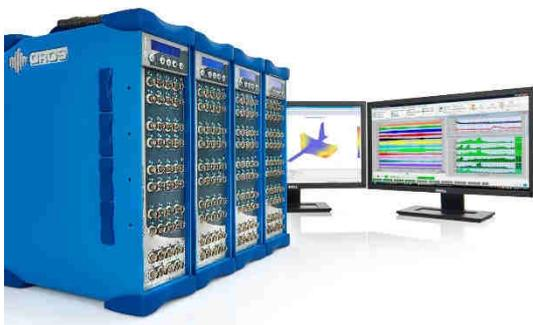
In the case of using several analyzers, the number of generators is multiplied by the number of systems and a high cross phase accuracy between units  $\pm 0.2^\circ$  is guaranteed.
