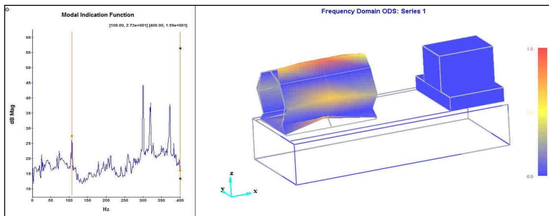
Fig3: ODS on a motor-pump unit
